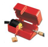
Avoid electrical accidents by applying lockouts to prevent plugs from being inserted into a wall outlet. Use when plug will not remain under the exclusive control of the person performing service or maintenance. Device is made of rugged engineering plastic and is designed for 250/500V electrical plugs. It Includes danger message printed on the device to alert workers of lockout program in progress. Can also be used to lockout air hose nipples.
